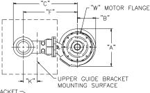
Note: 6" pump discharge can be connected to 5" or 6" flange.
