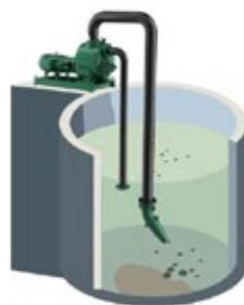
Vaughan Chopper Pump technology can also serve dry pit systems, delivering powerful mixing in below-grade or basement installations.
